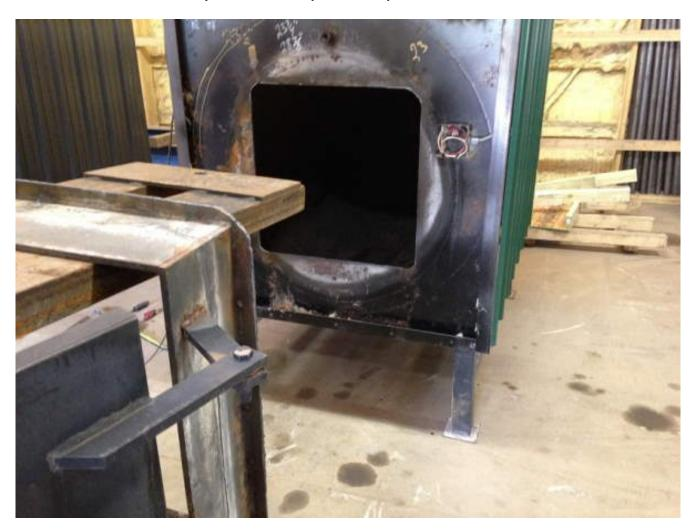
Then we cut the existing front plate out to the edge of the firebox.
