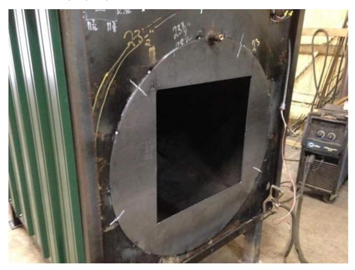
Then the door frame is reattached to the front of the stove. Again the previous measurements are used to insure exact realignment of the door frame. The frame is welded inside and out.
