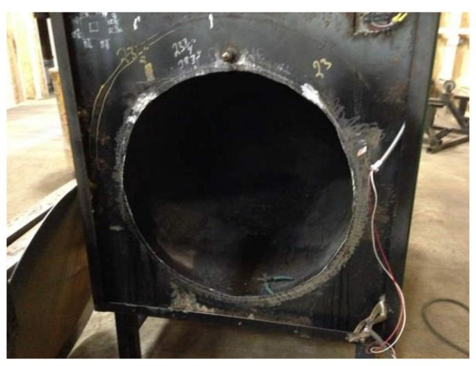
Next we attach a new plate to the front of the stove. The outside diameter is past the opening to allow welding inside and out. The door hole is placed based on the previous measurements to insure proper location on the door frame. We re-pressure test the stove to insure none of the welding has created any new issues and the stove is still properly sealed.
