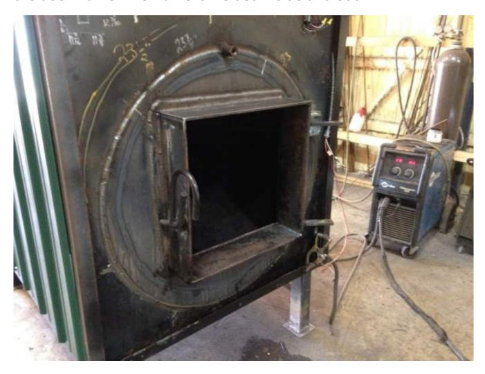
New angle is added for the barn steel, this angle is cut back to compensate for the door frame actually sticking out farther from the new plate. Everything is painted to prevent rusting.
